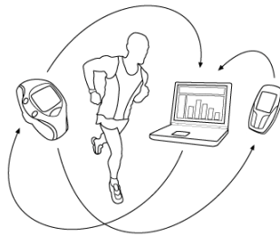
Fig. 2. An example of a multi-device system consisting of a wearable monitor (wrist unit), the desktop environment (a Web service and/or PC application) and a mobile application
